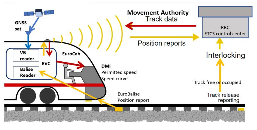
EVC automatically checks the permitted speed and brakes the train if necessary
