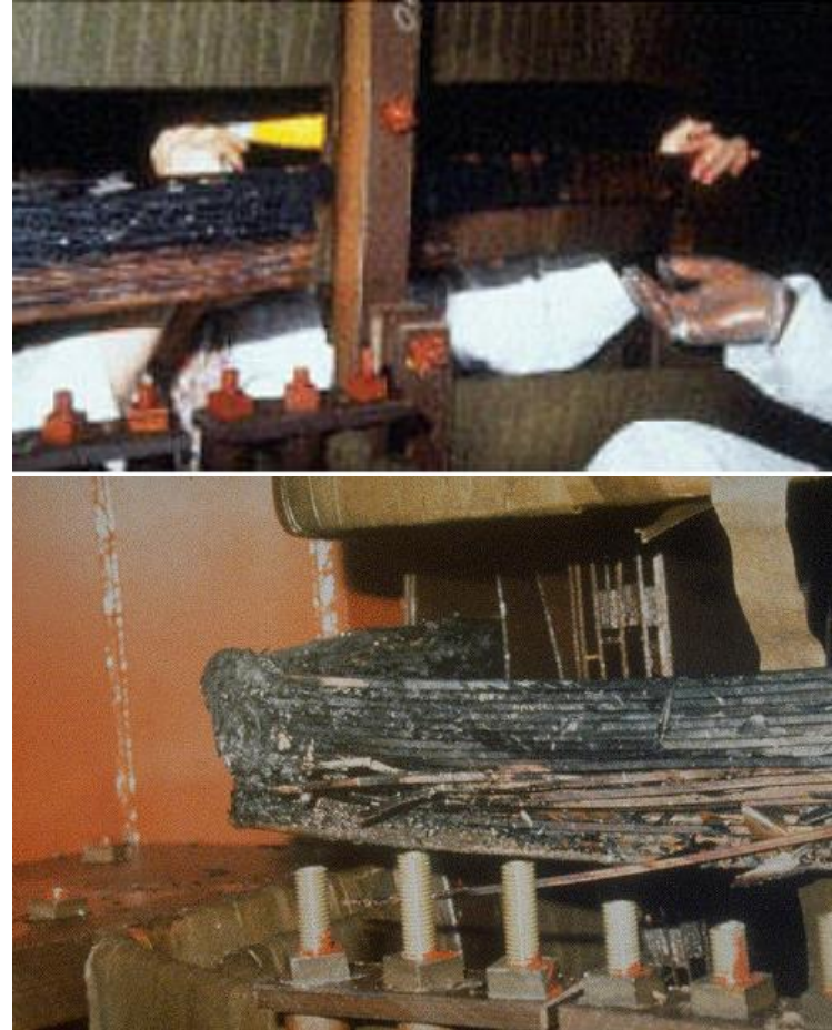
Salem Nuclear Plant GSU Transformer damaged by the GMD event of March 1989. (Photos courtesy of PSE&G.)
