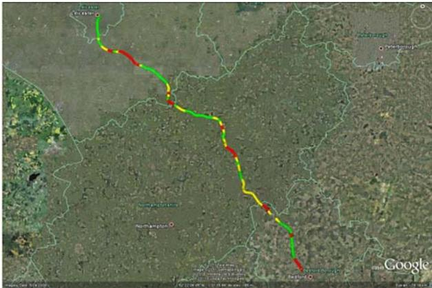
Figure 14. MODEM B (VODAFONE) SIGNAL STRENGTH INDICATOR (0-10 = Red, 11-20 = Yellow, 21-31 = Green)
