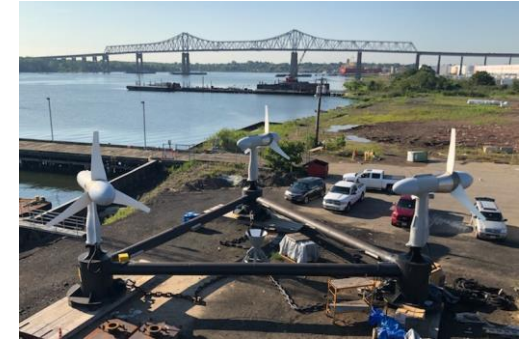
TriFrame™ Mount with Three KHPS Turbines
