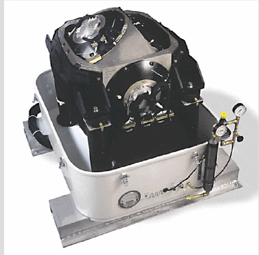
Gravity gradiometer: 350 kg+ http://www.ga.gov.au/image_cache/GA4750.pdf
