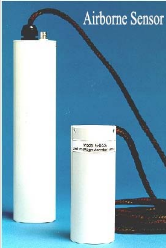
Geometrics G822 airborne Cesium magnetometer
