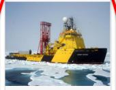
Combined Ice-breaker and AHTS suitable in harsh environment operations as well as the arctic
