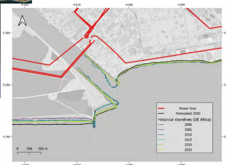
Coastal Erosion risk to the Power distribution system in Abidjan
